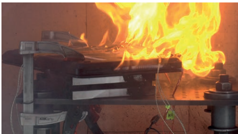
A laptop burns during the thermal runaway. © Fraunhofer EMI
