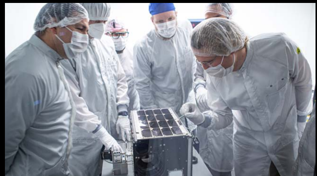
ERNST in the Fraunhofer EMI clean room: The research satellite was developed, integrated and qualified for space at Fraunhofer EMI.
