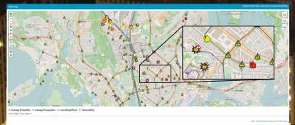
The picture shows a screenshot of the CAESAR software tool that allows for simulating cascading effects throughout different networks of coupled infrastructure systems. Here, you can see the results of a random power outage in Helsinki on water and communication networks.
